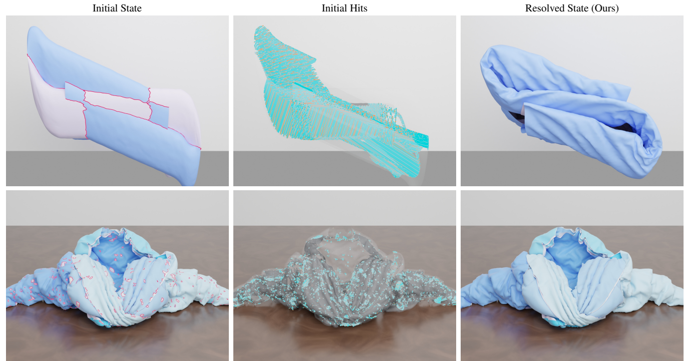
Fig. 1. Our self-intersection repair method resolves complex entanglements in thin-shell dynamics without topological classification. Top: A square cloth folds its corners inward, creating deep and nested self-intersections. Bottom: A complex garment drops onto the ground, concentrating thousands of intersection contours. By optimizing geometric separation directions directly, our algorithm achieves robust intersection repair, enabling practical, scalable simulation in highly complex intersection scenarios.
